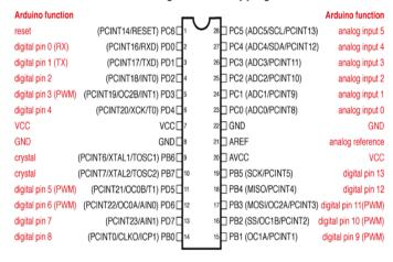
Digital Pins 11,12 & 13 are used by the ICSP header for MOSI, MISO, SCK connections (Atmega168 pins 17,18 & 19). Avoid low-impedance loads on these pins when using the ICSP header.
