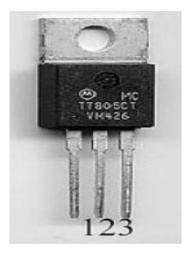
Pinout of the 7805 regulator IC Fig.3
