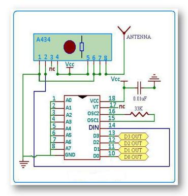
Fig.6-Block Diagram of IC-Decoder
