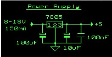
Fig.2-Circuit diagram of the power supply
