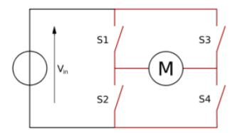
Fig.7-Structure of an H bridge (highlighted in red)
