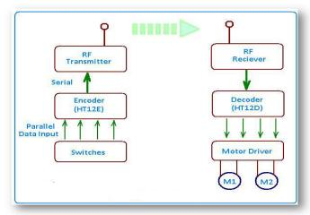
Fig.4-Block Diagram of RF Module
